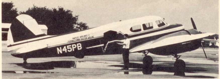
Step door, new rudder and fin, longer nose gives famed Cessna aircraft new appearance. Cabin modified to take six seats in Bay State conversion
